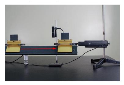
The glider then bounces off the sensor and passes through the photogate again. In an experimental run, you should record the two photogate velocity readings and the force-versus-time curve from the sensor.
