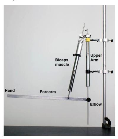
Two tension-compression gauges are employed to determine the compression of the humerus bone and the tension in the biceps muscle as various weights are placed in the "hand" (i.e., hung from the end of the forearm). The point at which the biceps muscle connects to the forearm can be changed,
