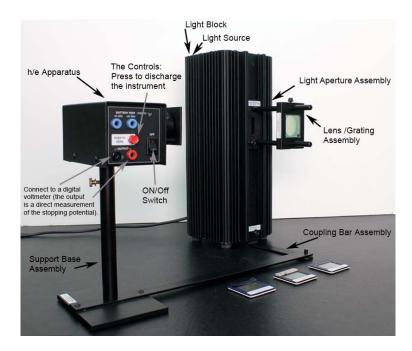
The equipment consists of a mercury vapor light housed in a sturdy metal box, which also holds the transformer for the high voltage. The transformer is fed by a 115-volt power source from an ordinary wall outlet. In order to prevent the possibility of getting an electric shock from the high voltage, do not remove the cover from the unit when it is plugged in.
