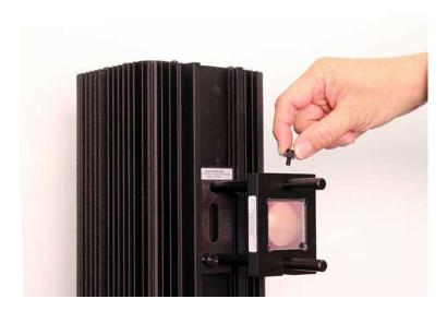
The variable transmission filter consists of computer-generated patterns of dots and lines that vary the intensity of the incident light. The relative transmission percentages are 100%, 80%, 60%, 40%, and 20%.
